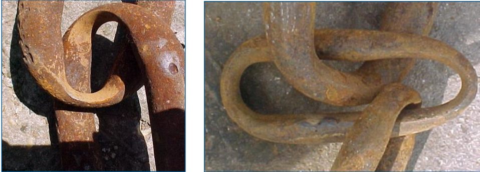
Figure 21 Abrasion and wear on mooring chains
