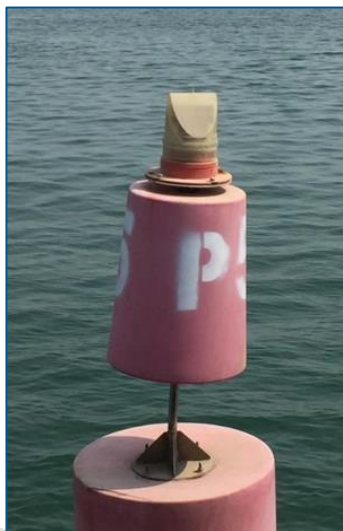
Figure 9 High Ultraviolet effect on red buoy
