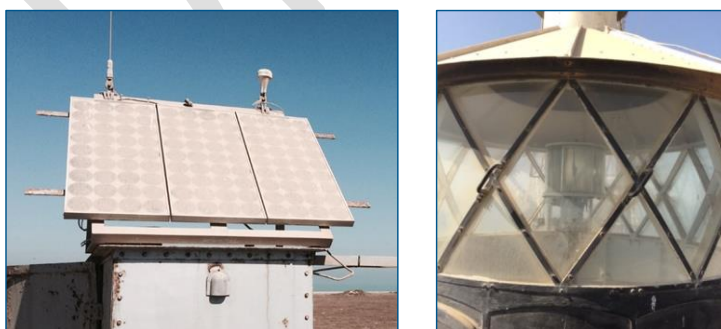
Figure 17 Presence of dust on AtoN device
